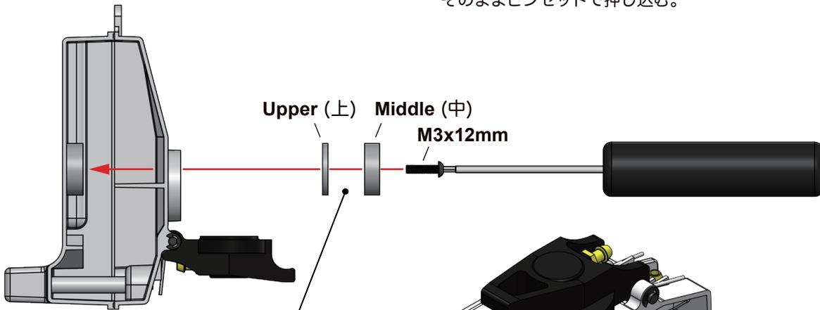
Place the Upper & Middle Fuel Tank Spacer onto M3x12mm Button Head Screw, Hold Fuel Tank lay down, Attach to the mounting boss.
