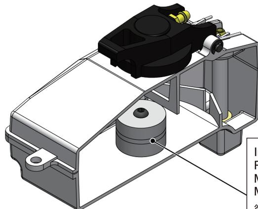
In case small adjustment, Remove Fuel Tank Spacer Middle 0.5cc (Change to M3x10mm Button Head Screw.)
